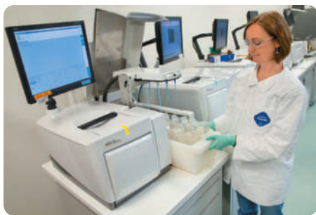
▲ The sequence of the approximately 5.8 billion nucleic acid units, or nucleotides , present in the human genome has been determined using instruments like this automated DNA sequencer.
